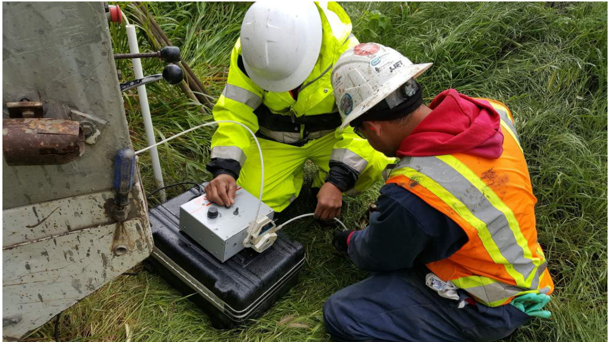
Photo 8: View of groundwater sampling in progress at SB-5.
