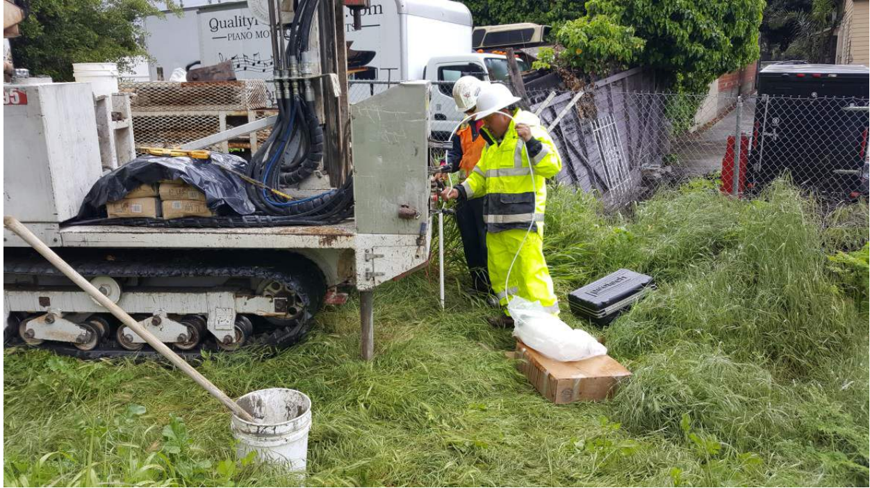
Photo 7: View of temporary well casing being inserted into SB-3 in preparation for collection of groundwater sample, looking south.
