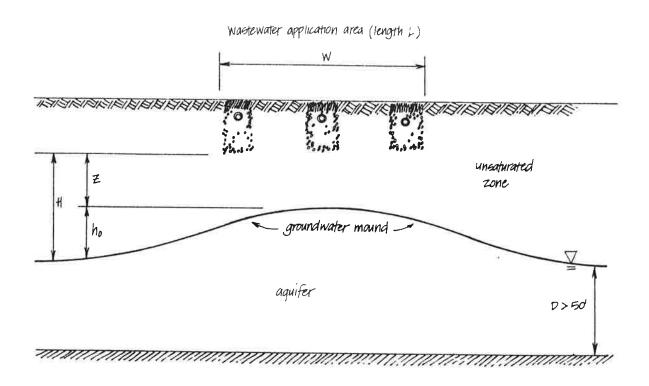
Fig. 2. Groundwater Mounding for Case 1 -Aquifer of Relatively Large Thickness
