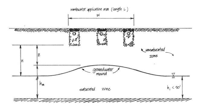
Fig. 4. Groundwater Mounding for Case 2 - Relatively Thin Groundwater Zone
