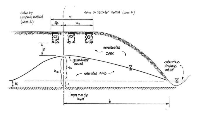
Fig. 7. Combined Application of Case 2 and Case 3 Methodologies
