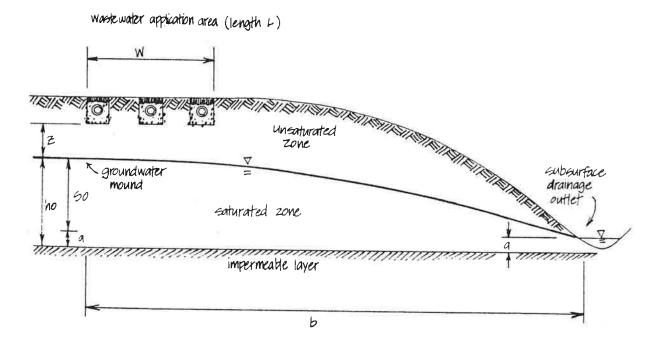
Fig. 5. Groundwater Mounding for Case 3 - Flow to Lateral Seepage Outlet
