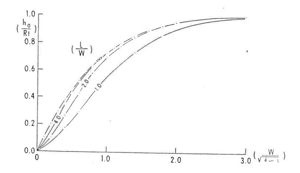
Fig. 3. Dimensionless Plot of the Rise at the Center (h<sub>o</sub>) of the Mound Beneath a Rectangular Recharge Area for Different Ratios of Length to Width (Glover,1966)
