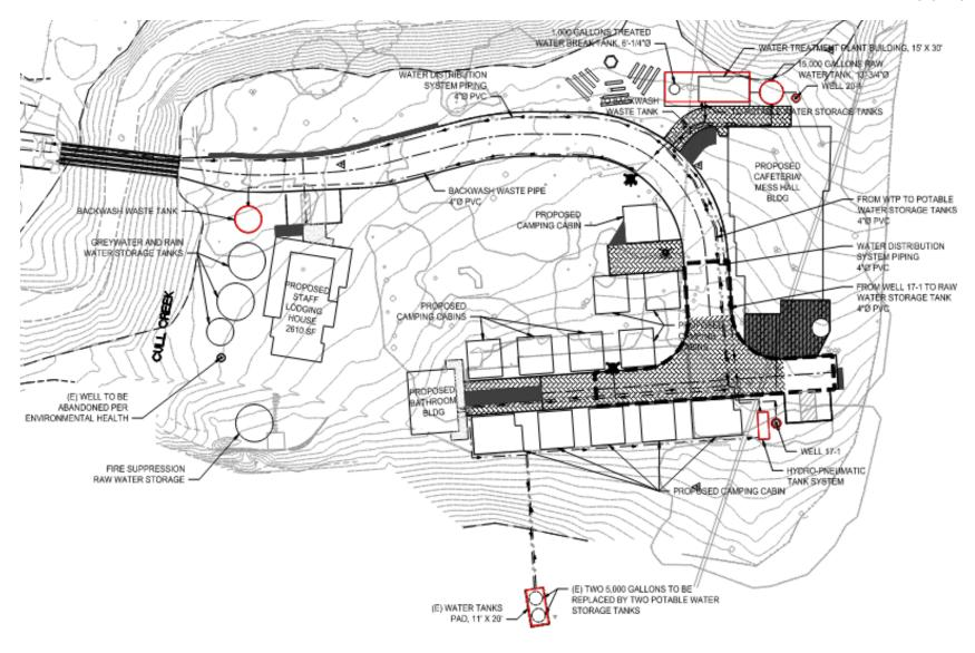
Figure 2 Water System Facilities Proposed Locations
