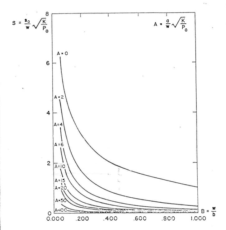
Figure 6. Subsurface drainage design graph.
