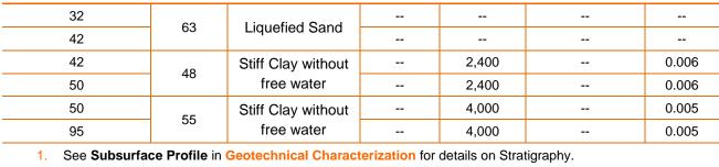
2. Parameters assume groundwater is located at a depth of 25 feet below the existing ground surface.
