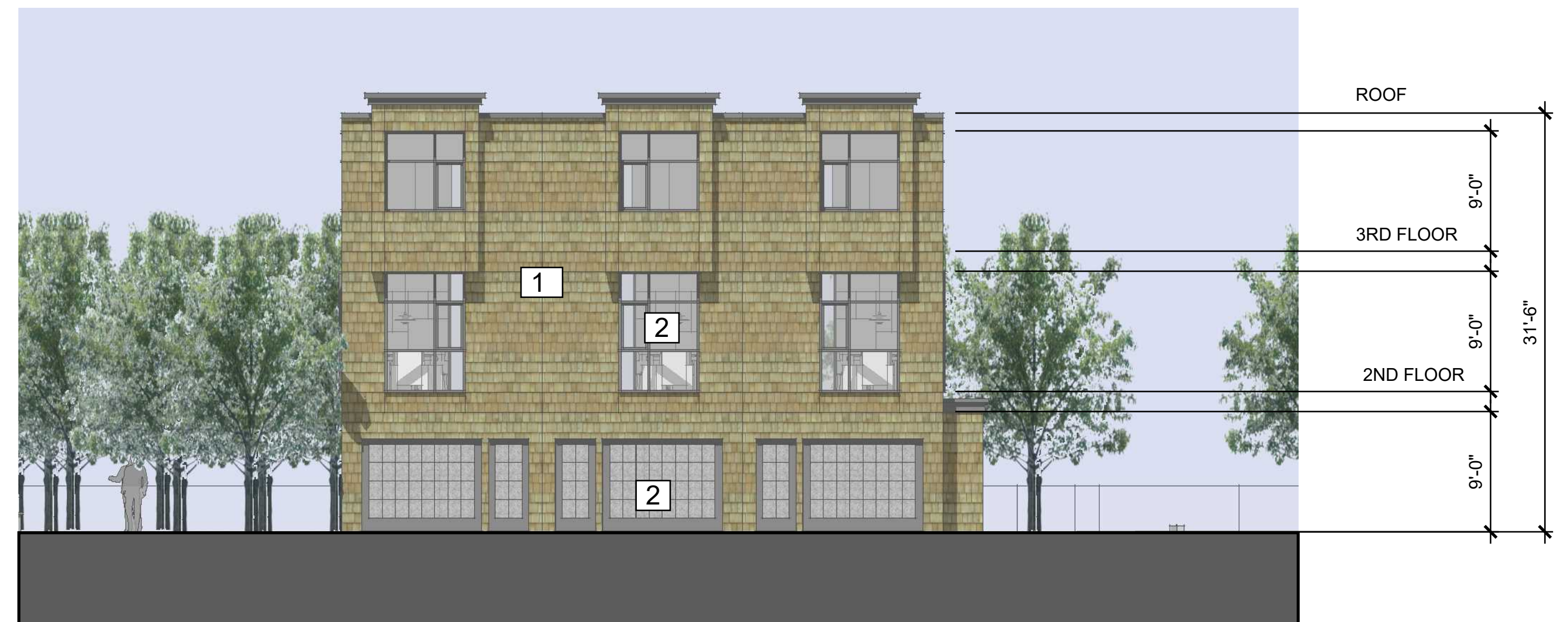
BLDG 5: REAR ELEVATION (BLDGS 1-4 SIMILAR)
