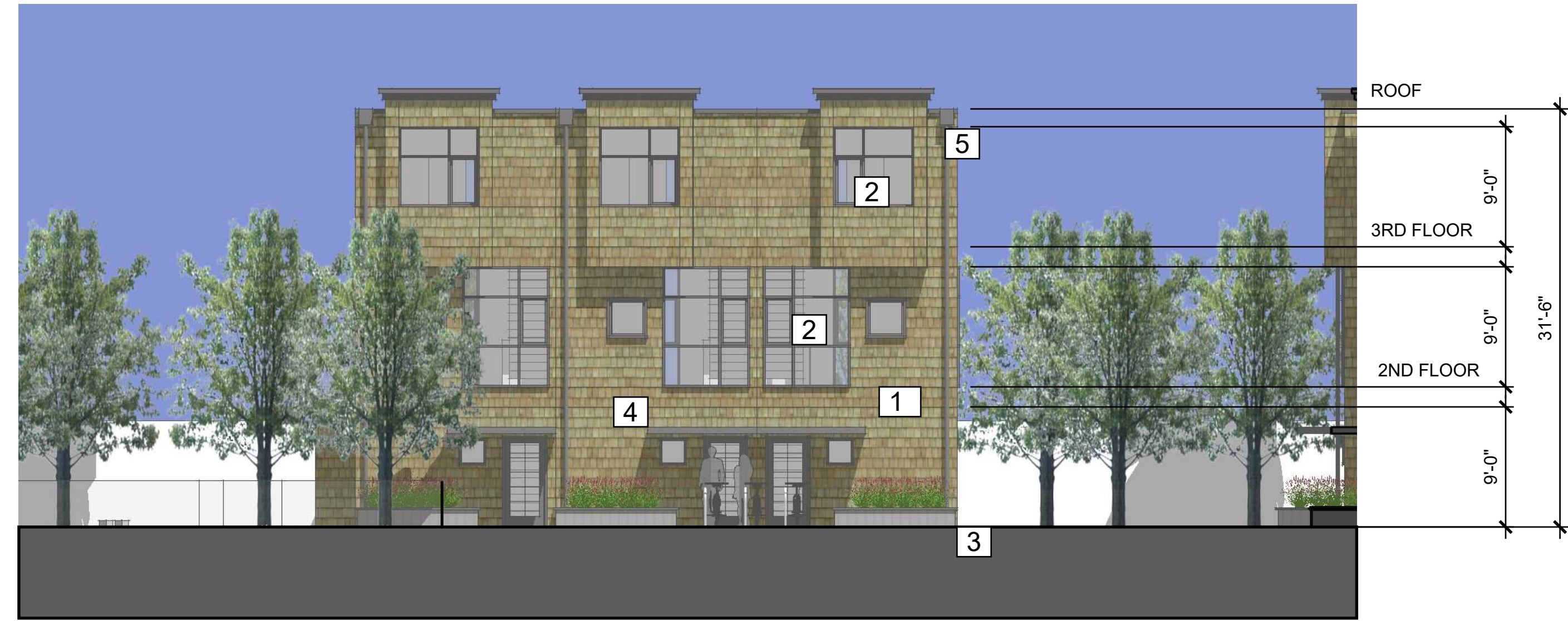
BLDG 5: FRONT ELEVATION (BLDGS 1-4 SIMILAR)
