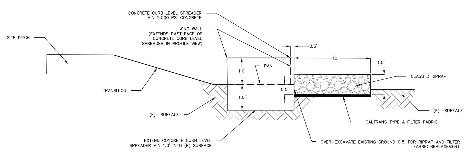
DETAIL 7 - LEVEL SPREADER PROFILE VIEW NOT TO SCALE
