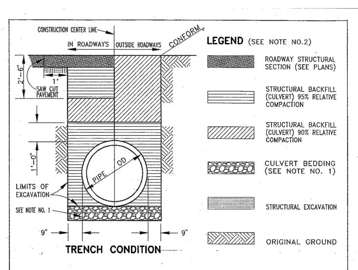
1. EXCAVATE UNSUITABLE SUBGRADE BELOW THE LIMIT OF EXCAVATION AND REPLACE WITH CULVERT BEDDING MATERIAL, ONLY IF SO DIRECTED BY THE ENGINEER. OVER EXCAVATION DUE TO FAILURE OF THE CONTRACTOR TO MAINTAIN SUBGRADE SHALL BE REPLACED WITH CULVERT BEDDING AT THE CONTRACTOR'S EXPENSE.
