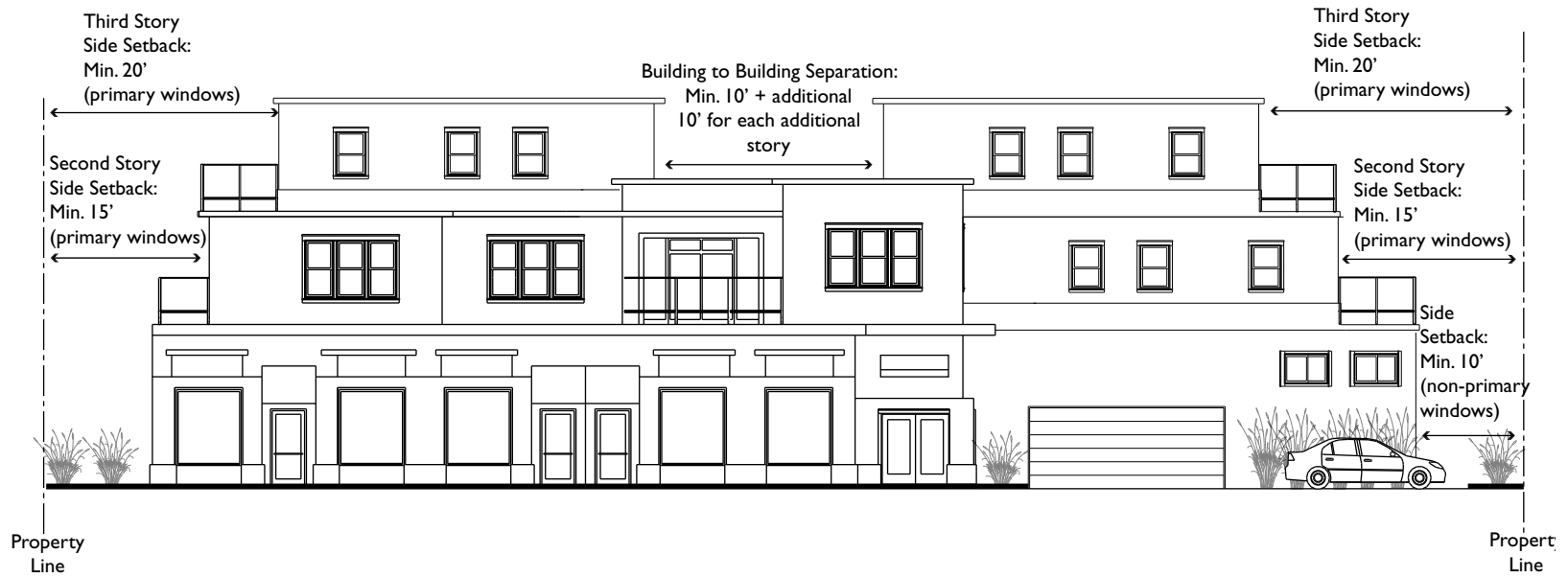
Figure 4.2-3: Residential Mixed Use: Setbacks for Primary Windows
