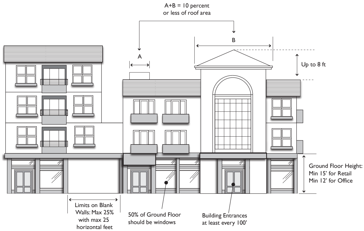
Figure 4.2-11: Residential Mixed Use: Height Projections and Façade
